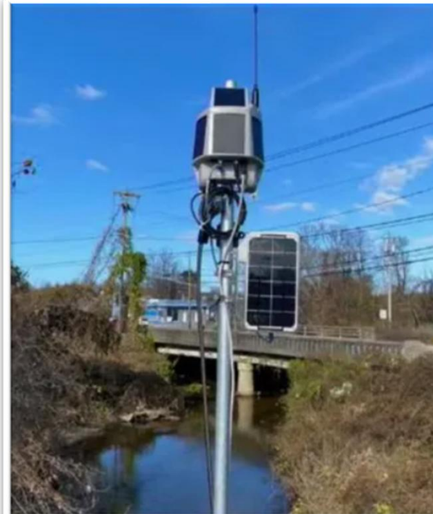
One of the AWARE Flood Sensor from Intellisense that Hendersonville now has around the city. These sensors use radar to detect water levels and automatically send updates to city staff. The blue part is the sensor, while the black part is the solar panel and battery that powers it. Public Document
